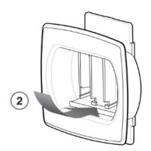
Continue pressing on the paddle until it rotates all the way in and locks into place.
